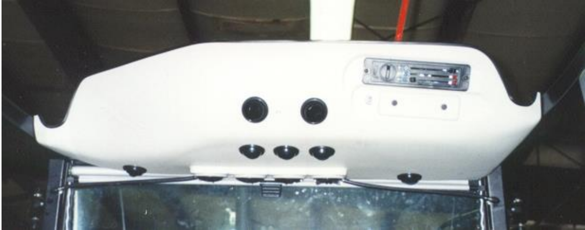
Louver arrangement with defrost louvers (optional) left and right at the windshield.
