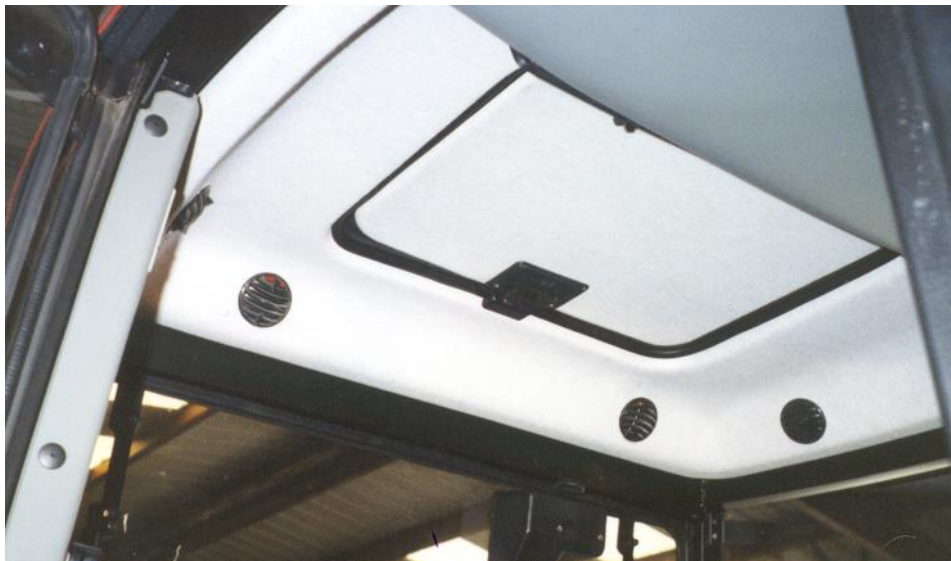
Rear recirculation louvers in place.
